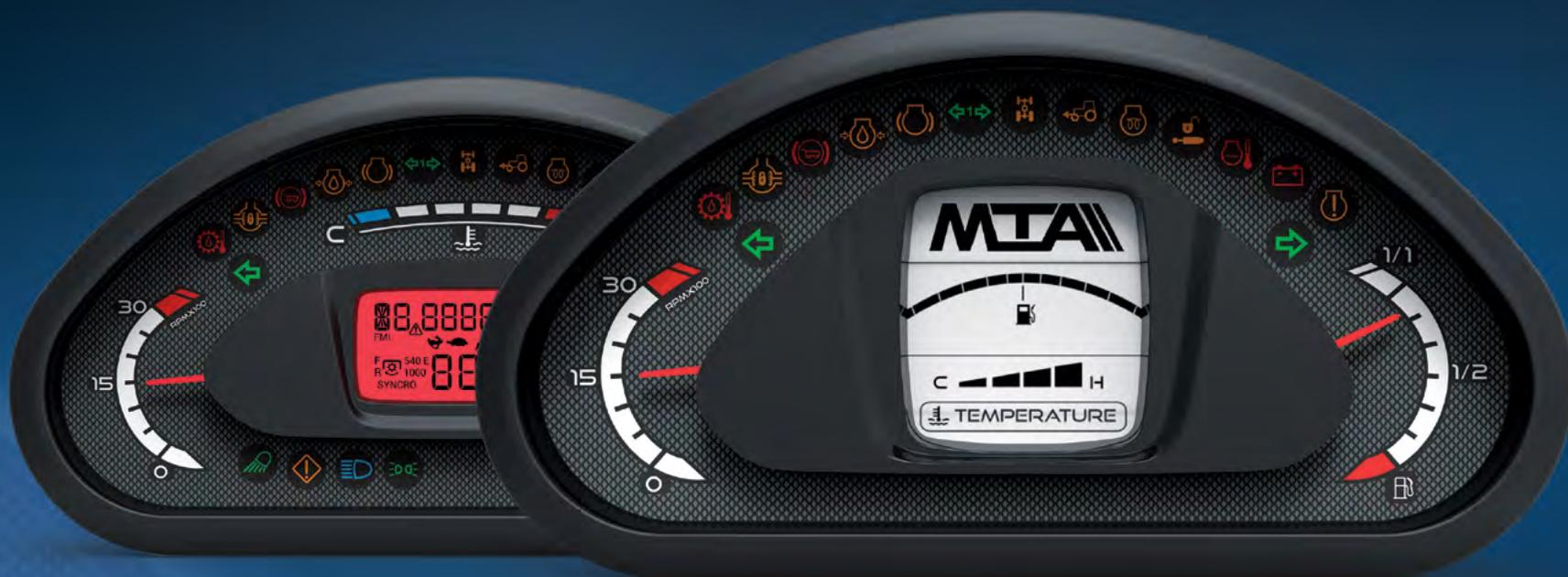
1 indicator with LED bar located above the display; 23 LED control lights; 1 real timer-clock; 1 buzzer; 1 CAN line with configurable terminal; up to 23 configurable digital inputs; 2 analogue inputs; 2 frequency inputs and 1 500mA output. The glass of the instrument panel is made from PMMA. Quik can operate at either 12V or 24V and the fixing system provides two possible options, with or without front frame.
