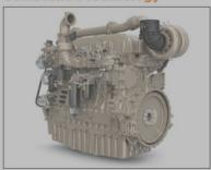
John Deere's new JD18 engine has a rated power range of 522 to 677 kW (700 to 908 hp). It features a rear gear train that optimizes direct power delivery while offering up to two rear auxiliary drives. It also features hydraulic lash adjusters for a maintenance-free valvetrain. Innovative combustion technology, which eliminates the need for aftertreatment systems, includes a simplified air system with fixed and wastegate turbos.
