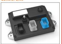
MTA announced a smart fuse box with an intelligent control unit that uses ST electronic fuses, the STi²Fuse. The unit is specifically developed for the off-highway industry and can be used to drive, protect, diagnose and monitor, through the STi²Fuse, up to 30 electric or electronic loads such as ECUs, ADAS systems, lights, heating, air conditioning and to interface analog/digital signals and loads via the vehicle's CAN network.
