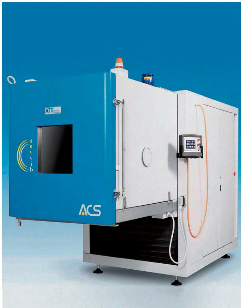
operating parameters of electromechanical components under testing, and was developed in collaboration with a leading company in the testing industry. We purchased a new thermal shock chamber and a climatic cell for environmental, thermal shock and vibration tests. This new equipment along with a vibration test bench enable simultaneous vibration and heat-cycle testing as well as the accurate simulation of the real-life operation of devices when installed in the vehicles.
