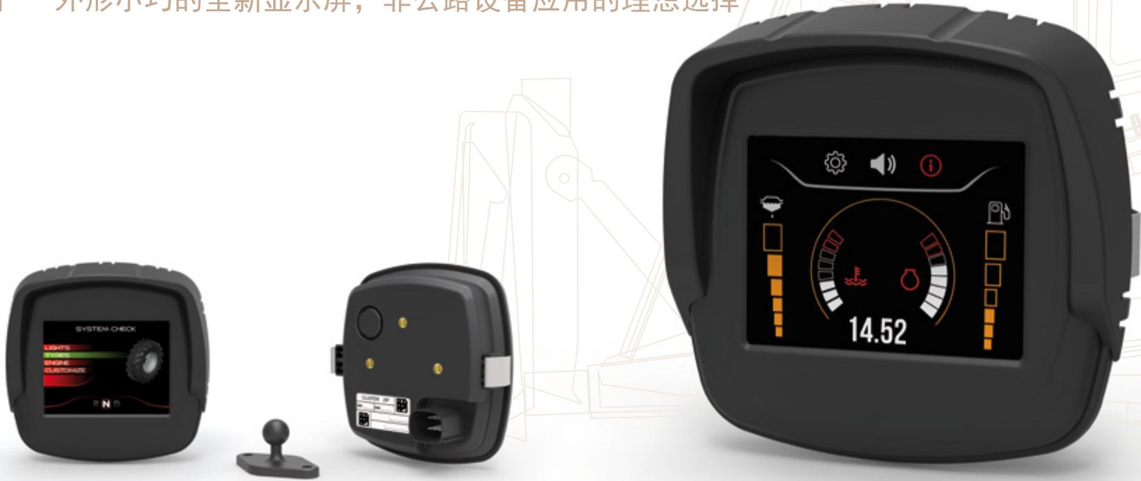
Zip is the latest display presented by our company within the range developed with the MTA Studio tool. It is a software developed by the electronics division with which the OEM can customize the display according to the uses of the machine on which it will be installed, and exploit this peculiarity to use the product on multiple vehicle platforms.
