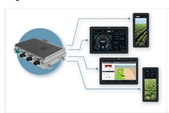
Agri SIC can be mounted on every cabin. It can handle up to 4 Full HD displays.
