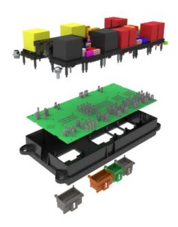
The fully customizable PCB is developed according to project needs. The fork type contacts used are assembled with press-fit technology, as well as the output connector tabs.
