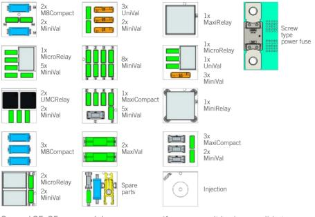
Several 35x35 mm modules with different contents can be positioned and oriented in the mold according to the customer's layout to obtain the required mask for the customized PDU.
