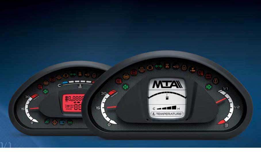
1 indicator with LED bar located above the display; 23 LED control lights; 1 real timer-clock; 1 buzzer; 1 CAN line with configurable terminal; up to 23 configurable digital inputs; 2 analogue inputs; 2 frequency inputs and 1 500mA output. The glass of the instrument panel is made from PMMA. Quik can operate at either 12V or 24V and the fixing system provides two possible options, with or without front frame.
