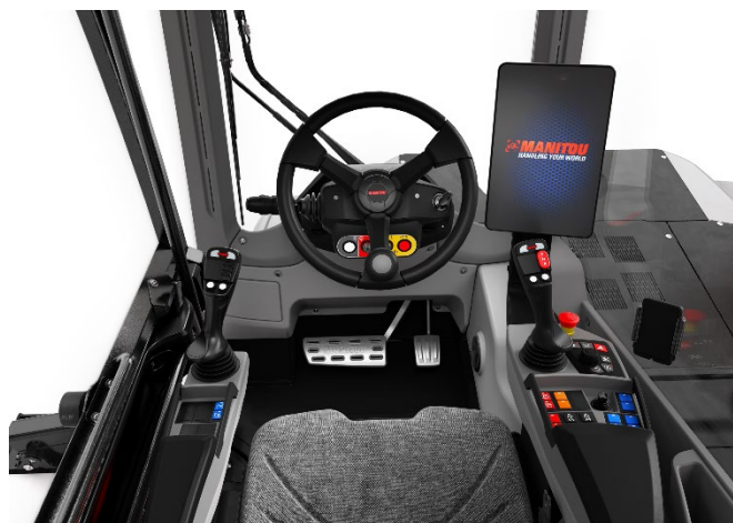
Leonardo display – in portrait mode - by MTA for Manitou MRT 2260 rotating telehandler
