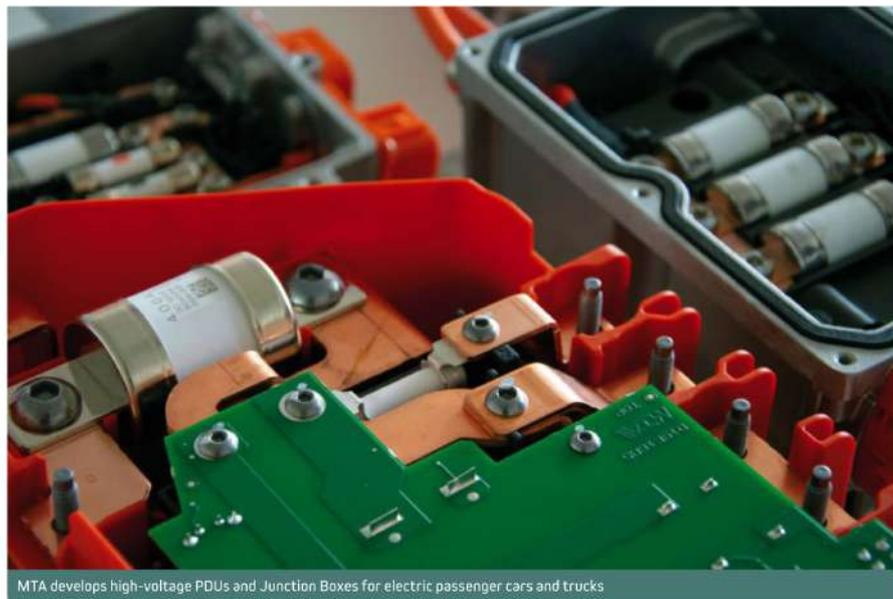
MTA develops high-voltage PDUs and Junction Boxes for electric passenger cars and trucks
