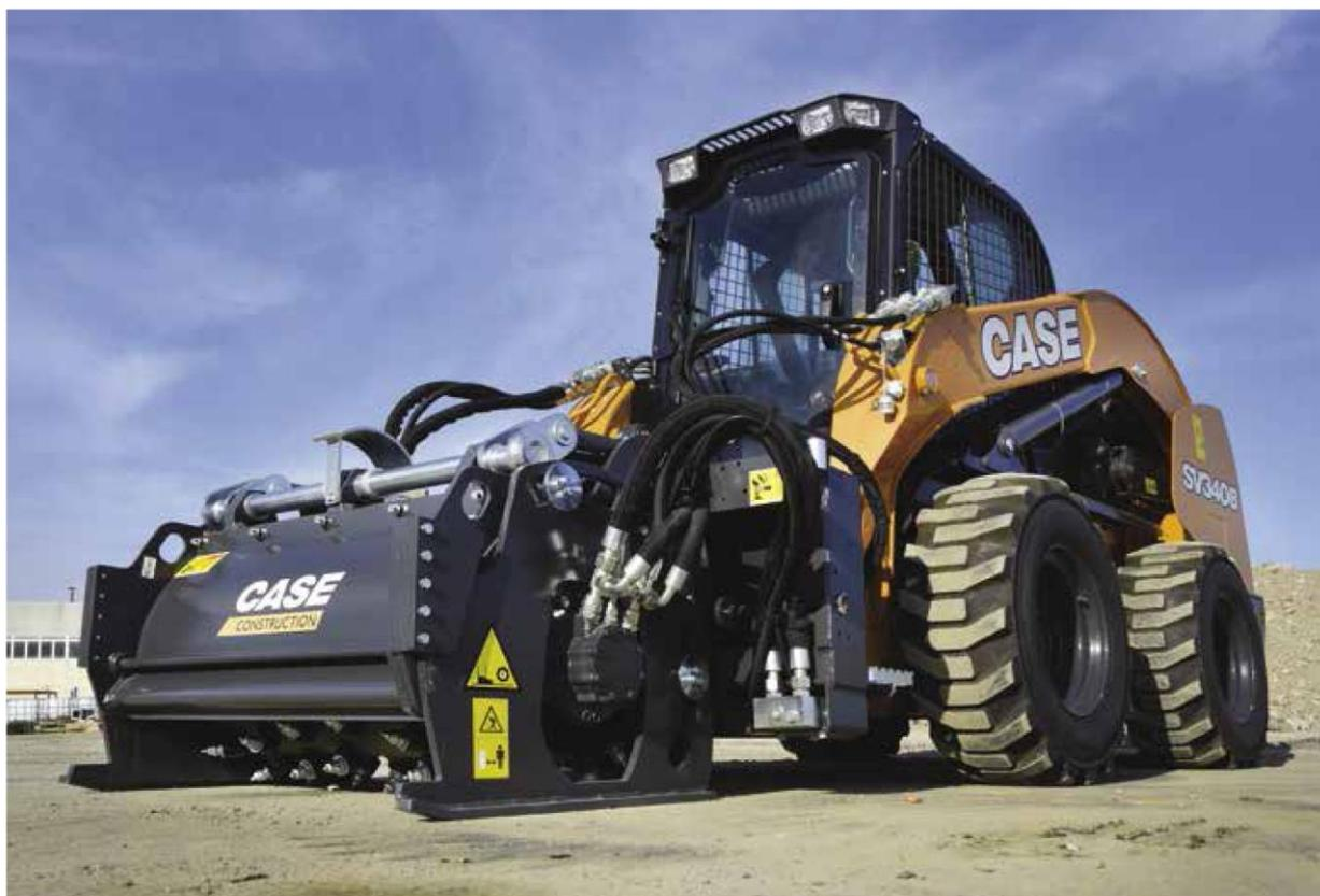
LA SERIE B DI CASE È DOTATA DI SISTEMI IDRAULICI AUSILIARI CHE POSSONO ESSERE AD ALTA PORTATA (HIGH FLOW) O AD ALTA PORTATA MIGLIORATA (ENHANCED HIGH FLOW), CON PRESSIONI FINO A 276 BAR, PER CONSENTIRE L'UTILIZZO DI ATTREZZATURE IDRAULICHE AD ALTA CAPACITÀ
