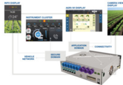
The “in-vehicle” system architecture. MTA S.P.A
