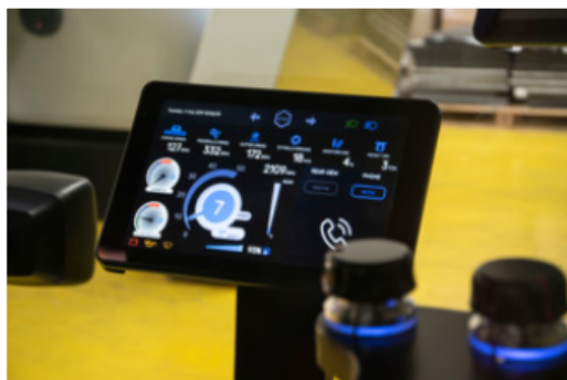
An MTA 12 in. multi-touch display which will be installed in the show cab.
