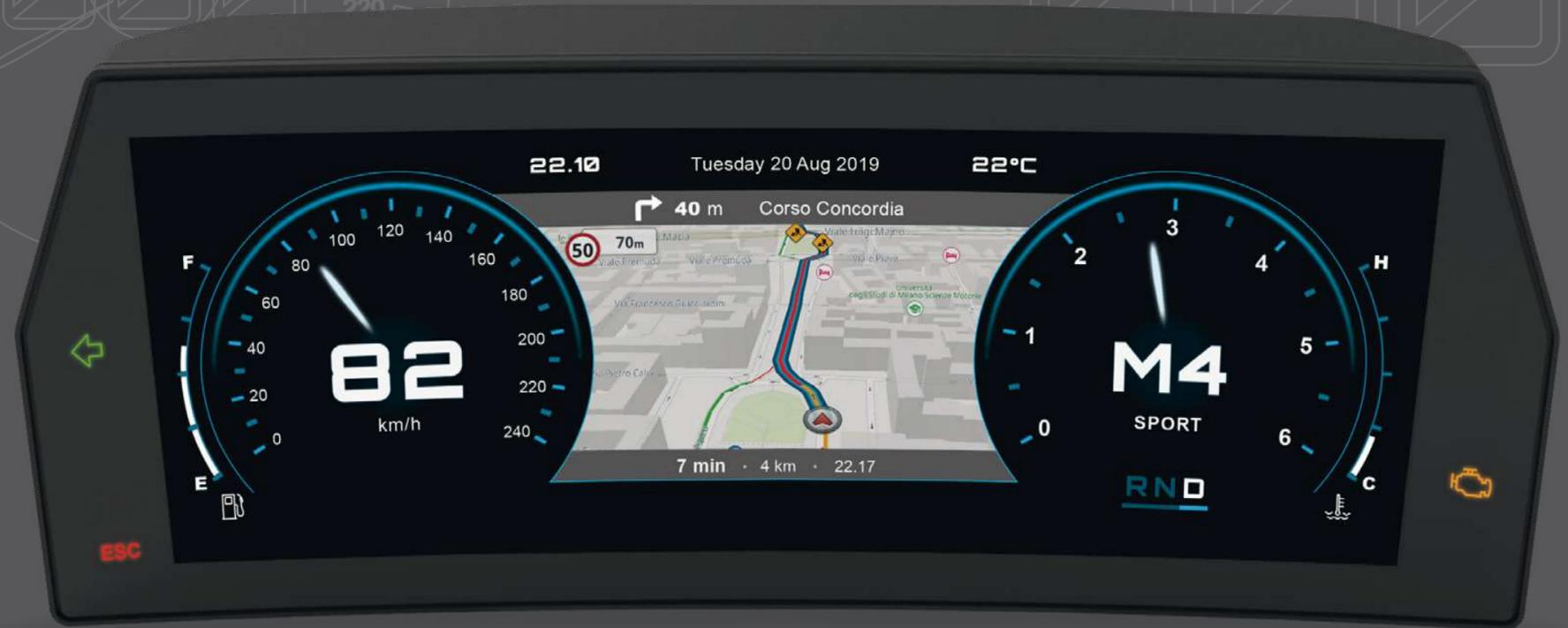
The current trend in the design of vehicle dashboards is oriented towards devices with highly customized geometries – even curved – with large dimensions and advanced graphics. A curve makes it easier for designers to create vehicle interiors with a greater aesthetic appeal than in the past, which enhances the vehicle and integrates perfectly with it. Ergonomics also benefits, improving legibility by maintaining the optimum distance between the image and the driver's eye.
